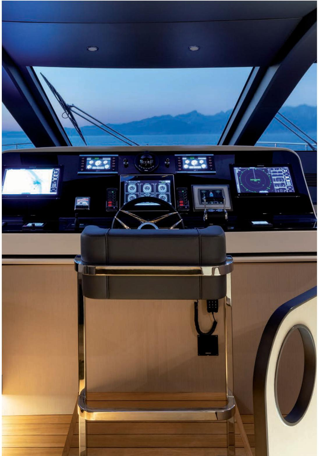
*Raised pilot house on an elevated half-deck between the main deck and the flybridge*
